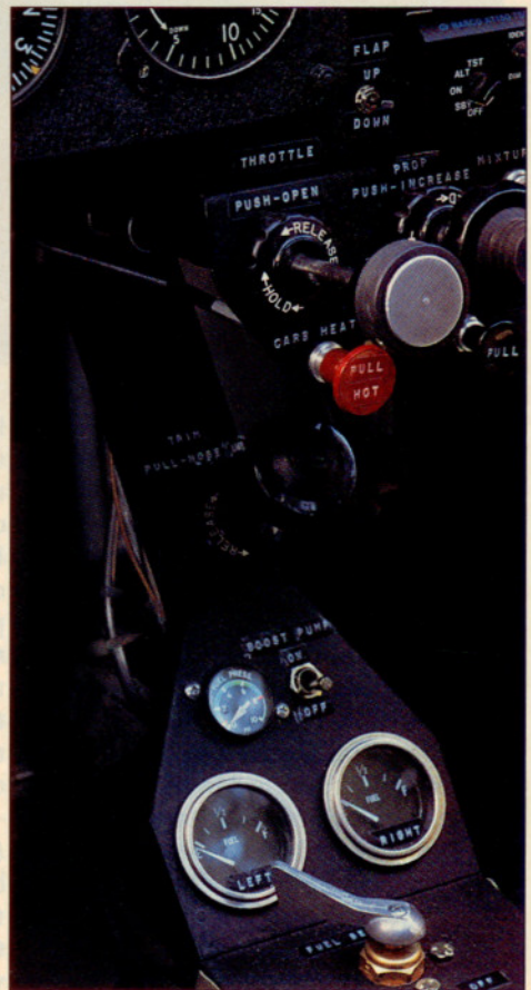
The RV's panel and sliding canopy (on the new -6T) highlight Van's reputation for efficient, conventional design. The fuel selector (right) clearly points to the tank in use.
